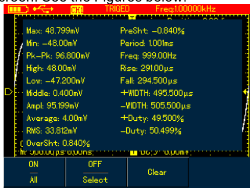
Figure 6-16A UTD1000CL measures all parameters
