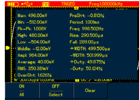
Figure 4-17A UTD1000CL measures all parameters
