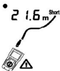
Figure 6.16 Short on Coaxial Cabling
