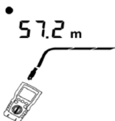
Figure 6.15 Open on Coaxial Cabling
